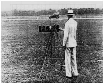
Figure: Greenshields measurement set up in the 1930s.
